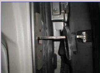
Reinstall bolts with a single drop of Loctite 242 (Blue)
