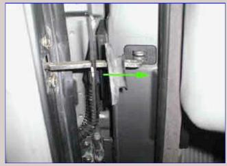
Install plate, then boot, then new hinge pin. Orient hinge pin so that locking tab faces outwards, to facilitate future removal.
