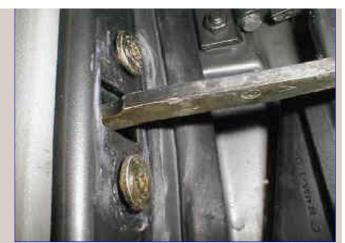
Place brake reinforcement over bolt holes in door. Straight edge faces interior of door, curved edge fits into curvature of door seal.
