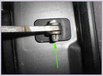
Lift boot on door upwards to disengage from to bolt, then pull downwards to disengage from lower bolt.
