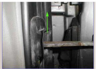
Boot is secured by sliding over the head of the door brake bolts.
