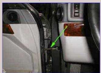
Locate locking tab on pin. Use a screw driver or punch to bend tab in.
