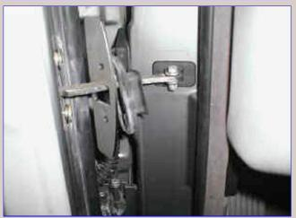
Remove both door brake retaining bolts. T30 Torx driver is required.
