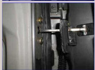
Place boot back over bolts by sliding onto lower bolt first, then upper bolt.
